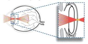
The laser beam passes through the clear cornea and lens implant. As the beam reaches its focal point on the cloudy capsule, the energy becomes highly concentrated causing disruption of the tissue and creating a tiny opening.
